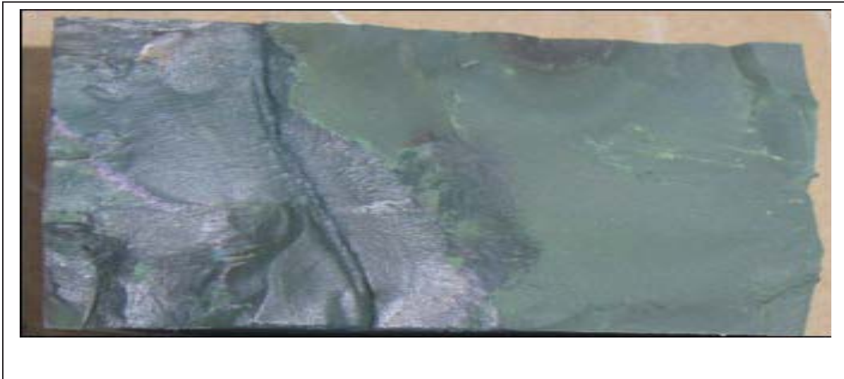
Figure 5-13: TOV Type Disk Failure Where a Preferential Path Failure Occurred (Arresterworks)
