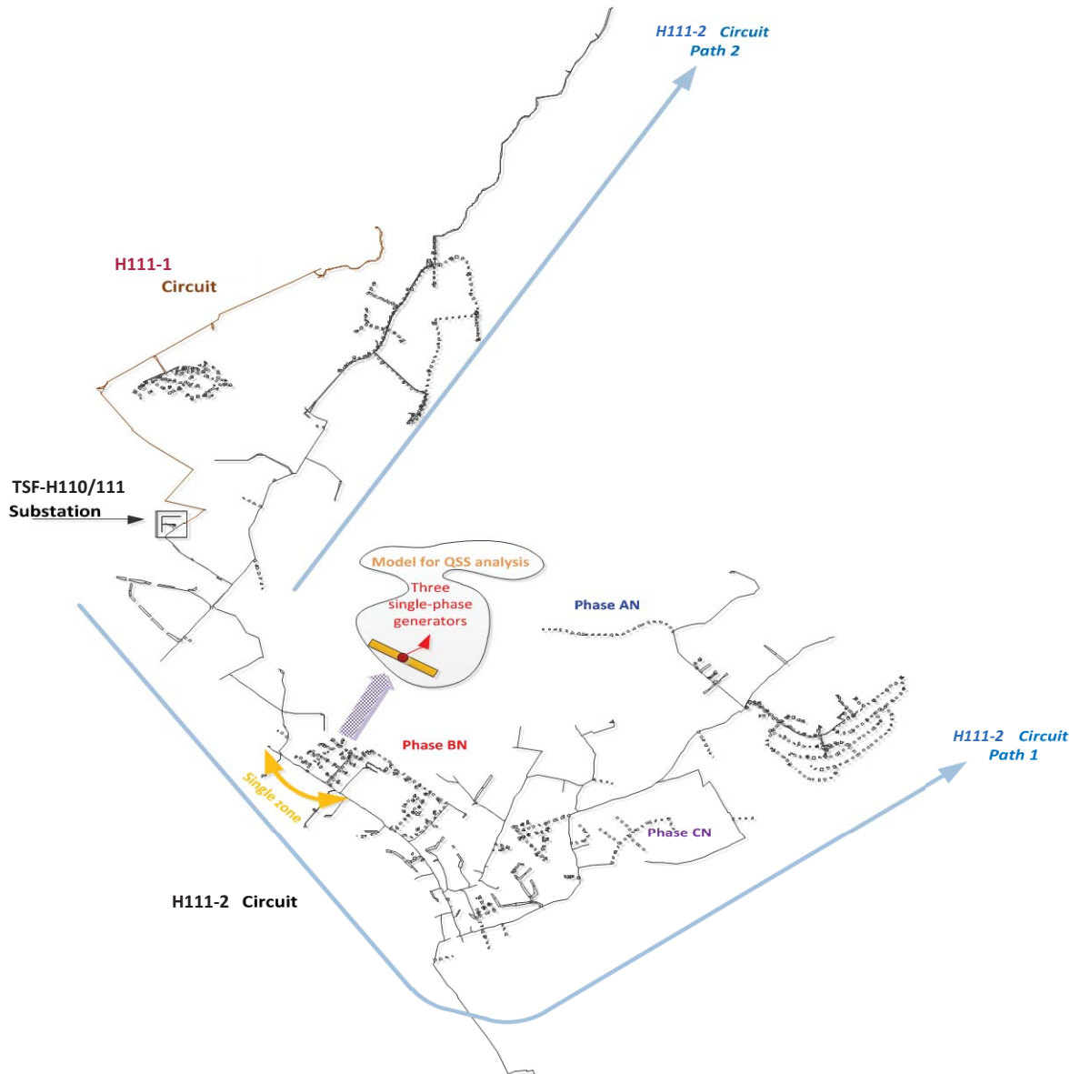
Figure 3-2: Demonstration of QSS Simplification of H111-2 Circuit
