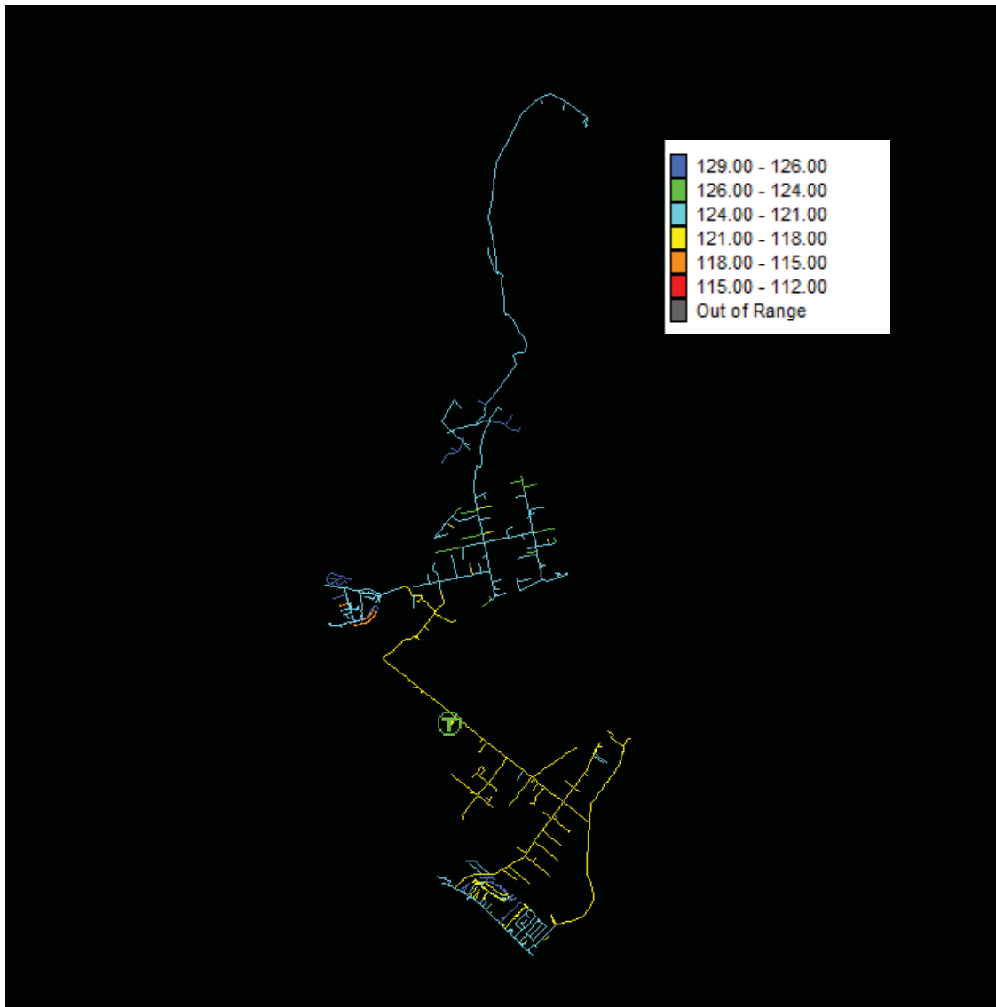
Figure 2-6. Min Load Scenario – Maximum PV Growth without FIT projects – Color by Voltage
